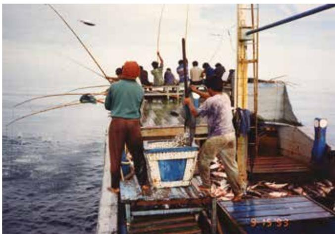
Picture 16. Live baitfish being transferred to a portable chumming tank on an Indonesian pole-and-line vessel (Photo: D. Itano)
