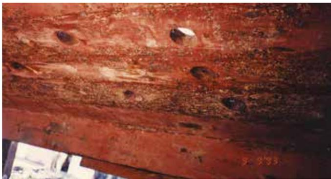
Picture 47. A simple method to enhance baitwell circulation is to drill holes through the hull to allow direct transfer of seawater to the open ocean (Photo: D. Itano)
