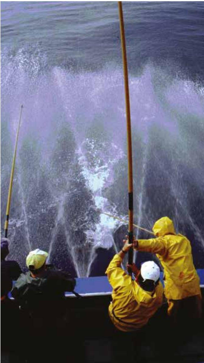
Picture 18. Seawater spray system on a Spanish Basque pole-and-line vessel (Photo: I. Onandia)
