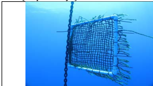
Figure 10.2. 1m x 1m plot of coir mesh deployed at U FAD, nearshore Kaneohe (left) and longline float with coir mesh wrap and tail deployed at Coconut Island, Kaneohe (right).
