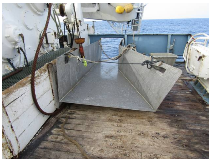
Figure 4. Ramp to release large bycatch, such as adult sharks, through the top deck door opening.
